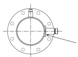
Before Welding, the base should be processed as the same as the circular arc of pipe to ensure sealing
