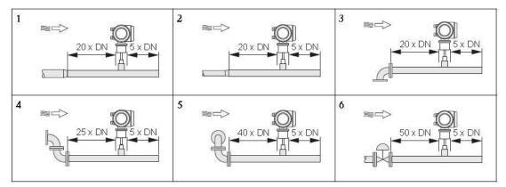
1 = Reduction, 2 = Expansion, 3 = 90° elbow or T-piece, 4 =  $2 \times 90^{\circ}$  elbow, 5 =  $2 \times 90^{\circ}$  elbow (3-dimensional), 6 = Control valve or pressure regulator.
