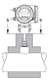
a Maximum insulation height for the flanged sensor
