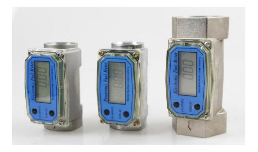
The diesel fuel can be used to measure the flow of water, methanol, urea, diesel, gasoline, etc. It provides highly accurate and durable performance, small volume turbine flow meter, and is designed with output module. The features of the display are, 2 accumulations, resetting and accumulating and optional unit conversion of Gallon and Liter. It is easy to change the spare parts inside, to maintain and assemble due to its compact design. Lithium battery can supply for 9000hours.
