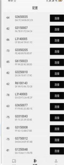
Select the device station address you need to configure, The station address is on the nameplate of the equipment shell.
