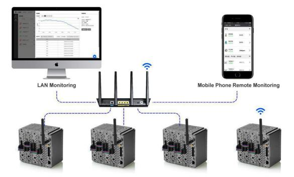
2. The combination of MLG020 host and MST530 series connects to the system via Ethernet (wifi)
